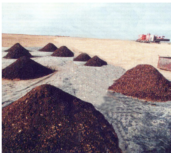
Figure 5 – Pilot project of oily waste composting
